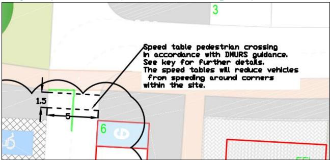
Figure 5-1. Speed Table Dimensions (60646100-AEC-GEN-L0-DR-CH-01\_000-P01.1)
